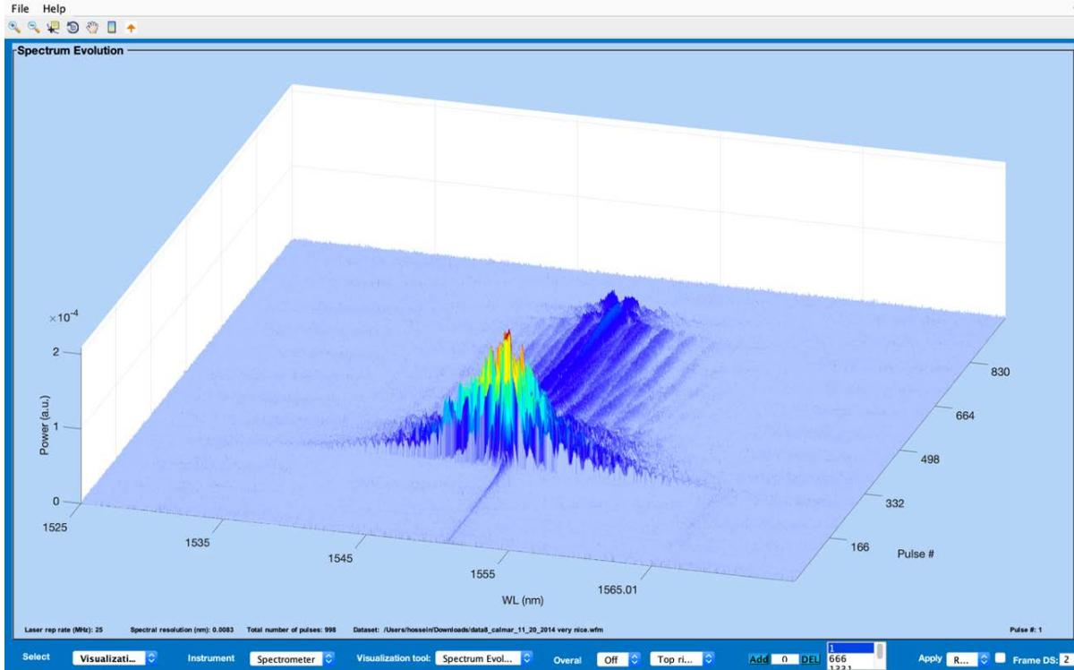
**20,000 Single-shot spectra of turn-on transients, Ti-Sapphire laser, captured at 90.8 Million frames/second.**
