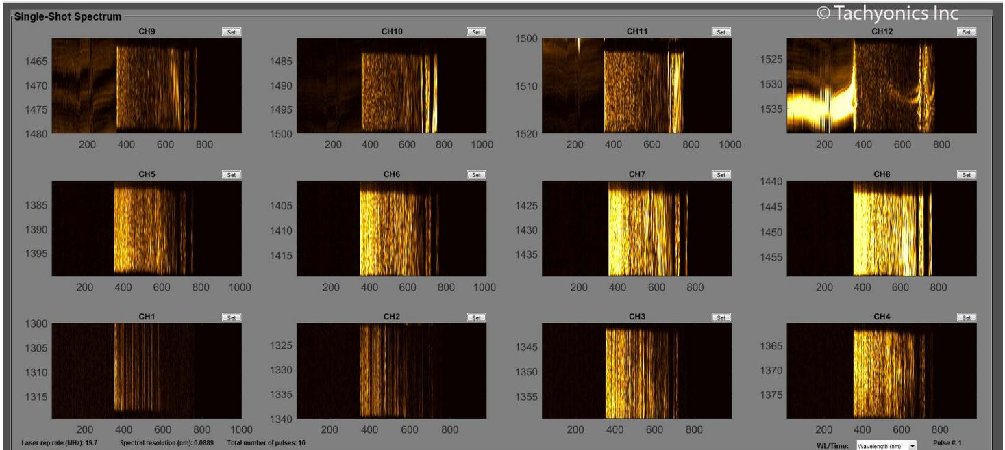
**Ultrafast Optical Coherence Tomography (OCT) imaging system enabled by COMET spectrometer: 720,000 single-shot consecutive line images at image acquisition speed of 36,000,000 lines per second.**
