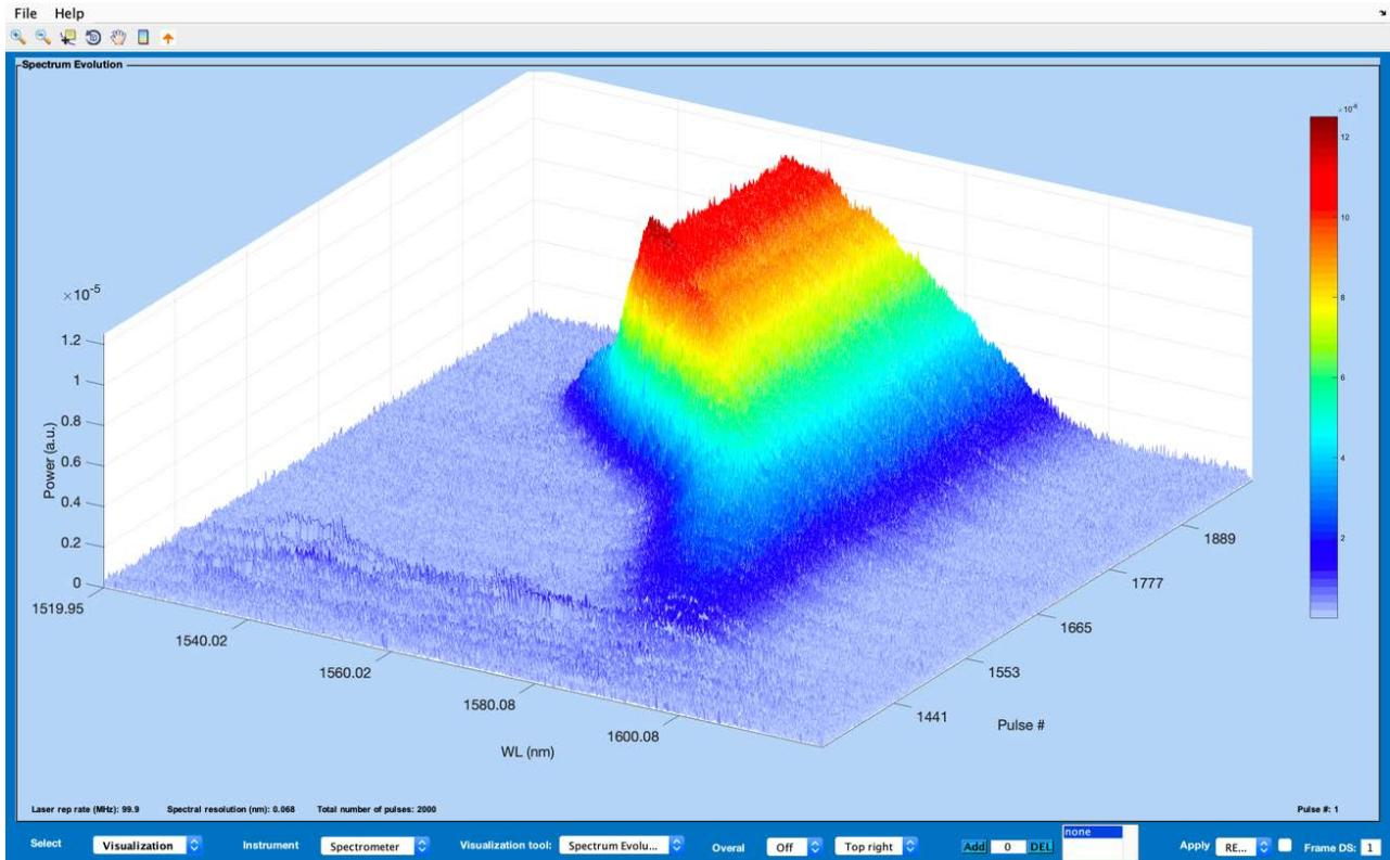
**COMET is showing effect of nonlinearity in an Optical Coherence Tomography (OCT) imaging system.**
