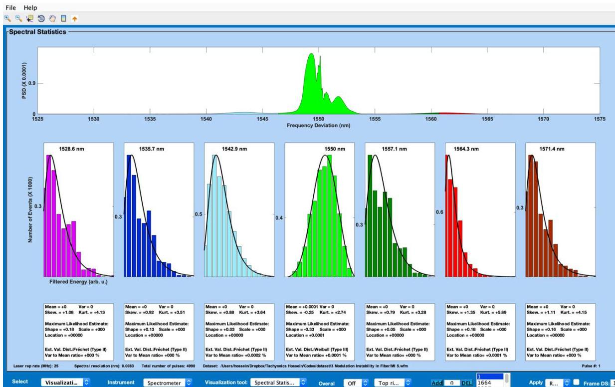
**12-probe ultrafast imaging/vibrometry system enabled by single COMET spectrometer:
